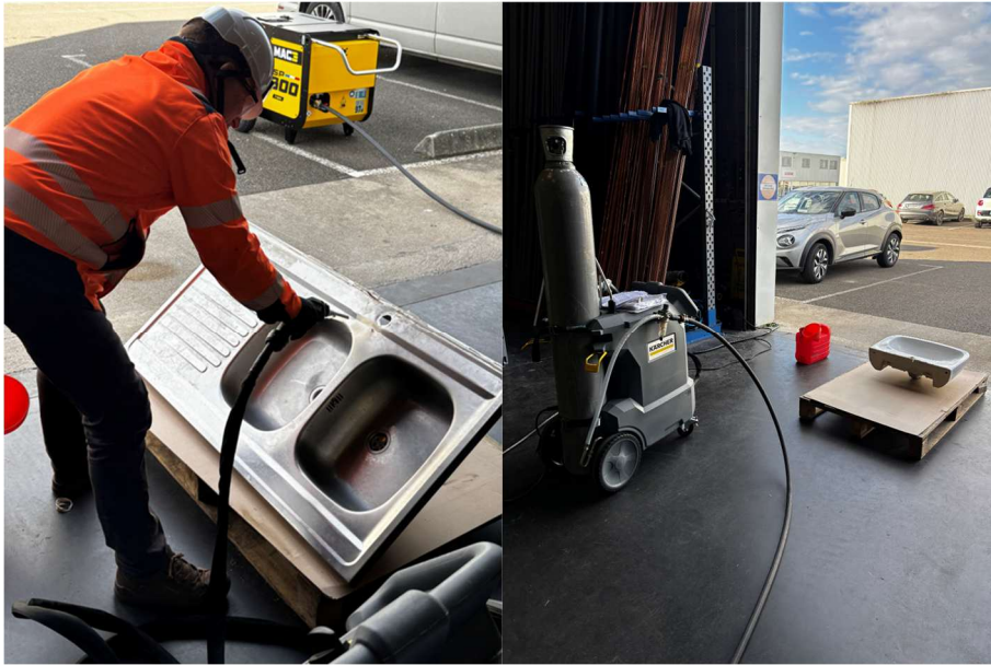
Figure 82 : testing the cleaning process for the reemployment of the sanitary equipment; @Favre
